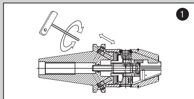
To adapt the drill chuck from the basic form to "Form B", the set screws have to be turned from their basic position into the borehole "B" by means of an Allen-“T“-Wrench SW 2,5.
