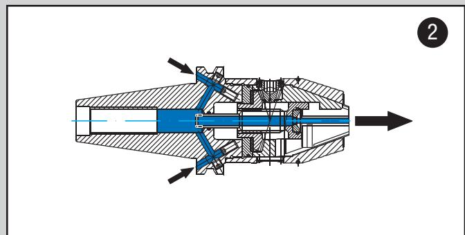
Consequently the set screws open the coolant supply through borehole “B” whereas the coolant feed from the machine is sealed by the pull stud.
