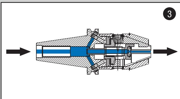
Adapting the CNC universal drill chuck to “Form AD” again the set screws have to be turned back to its basic position. Consequently the borehole “B” is blocked. The coolant feed from the machine is guaranteed by using a clamping bolt with a borehole.
