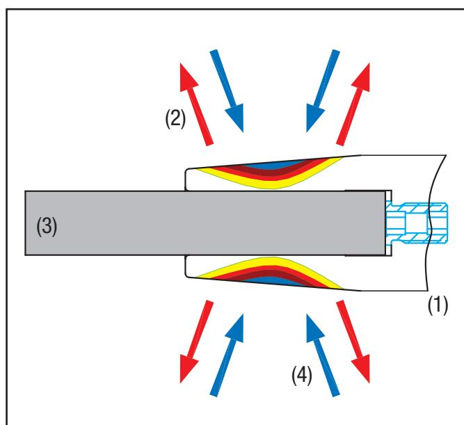
As the induction coil heats the shrink fit chuck, the chuck expands and the cool tool shank can be inserted. When the shrink fit chuck is cooled down again it contracts and forms a connection with force closure due to the oversize on the tool shank.
