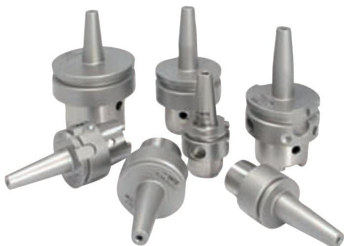
Our shrink fit chucks with axial length adjustment are used for metal and wood processing machines with rotating and static cutting tools. Shrinking technology makes use of thermally-related expansion for tool clamping. The application range of our tools goes for processes like milling, heavy-duty metal cutting, HSC milling, drilling, reaming, turning, wood machining or internal grinding.
